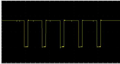
If your remote need negative signal, shortcut the X servo pin (yellow Square on the image) to ground pin (one of the black square pins on the image) and the signal will be reversed like this:
