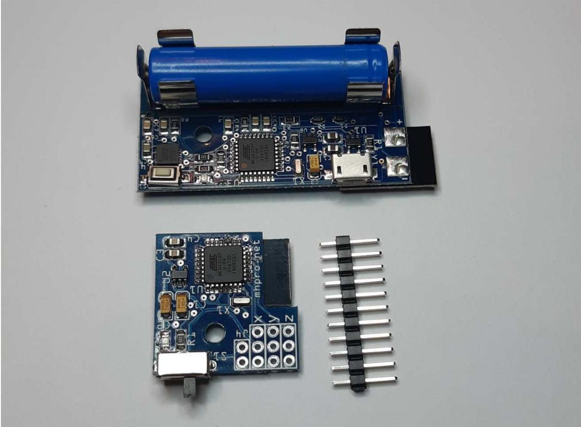
This 3 axis motion sensor gyroscope allows you to track the movement of the head or arm and replicate it to servos by the air (about 30 feet). For Do It Yourself (DIY) home project lover who dreams of doing a head tracking system FPV themselves cheaply.
