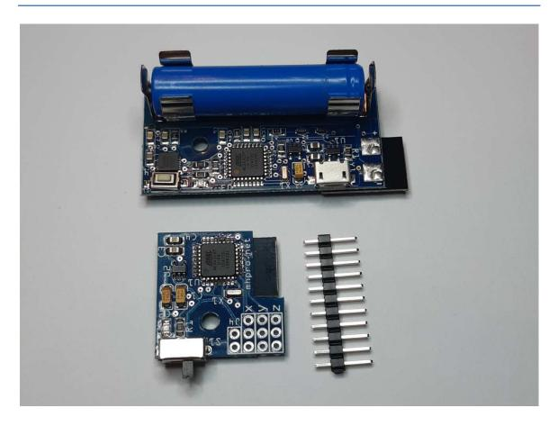
This 3 axis motion sensor gyroscope allows you to track the movement of the head or arm and replicate it to servos by the air (about 30 feet). For Do It Yourself (DIY) home project lover who dreams of doing a head tracking system FPV themselves cheaply.
