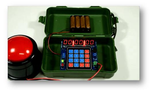
Trigger your switch to start the chronometer and to stop it. When the chronometer is stopped, you can reset it by pressing the « 0 » key. Otherwise, the time will continue from where it was.
