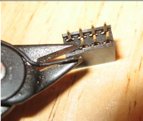
Cut the edge of the removed connector's tab.
